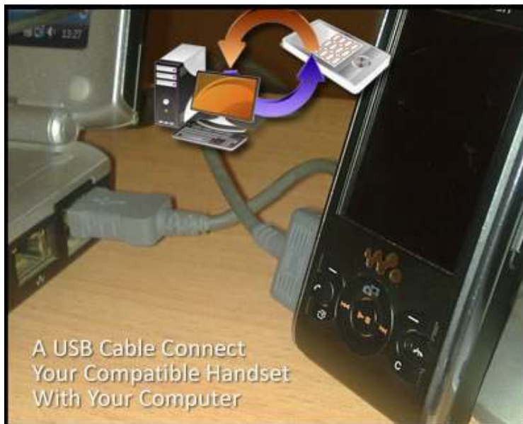
Figure 1 a typical setup of Text Processing System using SMS Spike and a Sony Ericsson Handset with a SIM Card. The number of the SIM card will be the service short code line
